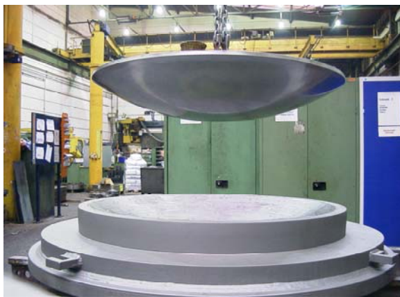
Fig. 3, 4: MAURER spherical bearing, installed MAURER Swivel Joist expansion joint
